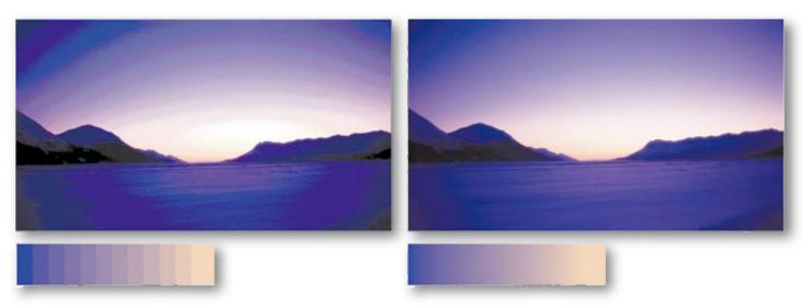
8 bit images can cause banding on subtle gradients. 10 bit images can render smooth gradients, at the cost of larger files and higher bandwidth.
